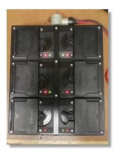
The PBR0406 battery charger is specifically designed to charge the PBR0406 battery.
