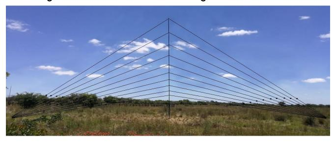
The BILP2514 is a wideband, high power HF Log Periodic antenna, optimised for short (NVIS) and medium range communication. The antenna that exhibits an omni-directional, high take-off angle, high gain radiation pattern ideal for NVIS communications links.
