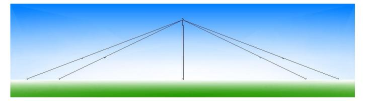
The BDA1000 is a HF Wideband Dipole Antenna designed for use in the base station and stationary mobile communications role.
