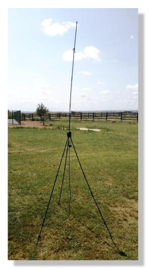
The BFT30-88 is man-portable VHF omni-directional antenna, designed for extended range VHF man-pack transceiver communications.
