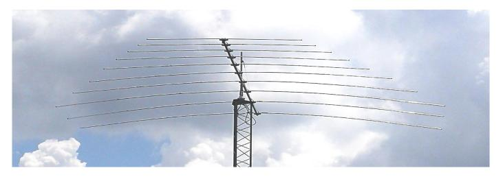
The BLP10-30-8 is a high gain, directional antenna designed for use in the permanent/strategic base station role. Manufactured from aluminium, UV resistant thermoplastics and stainless steel hardware to ensure durability and long service life.
